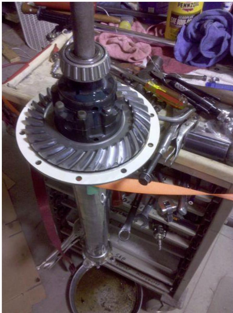
Then I installed the bells and put a dab of sealant on each bolt. And put it all together for the final time.
