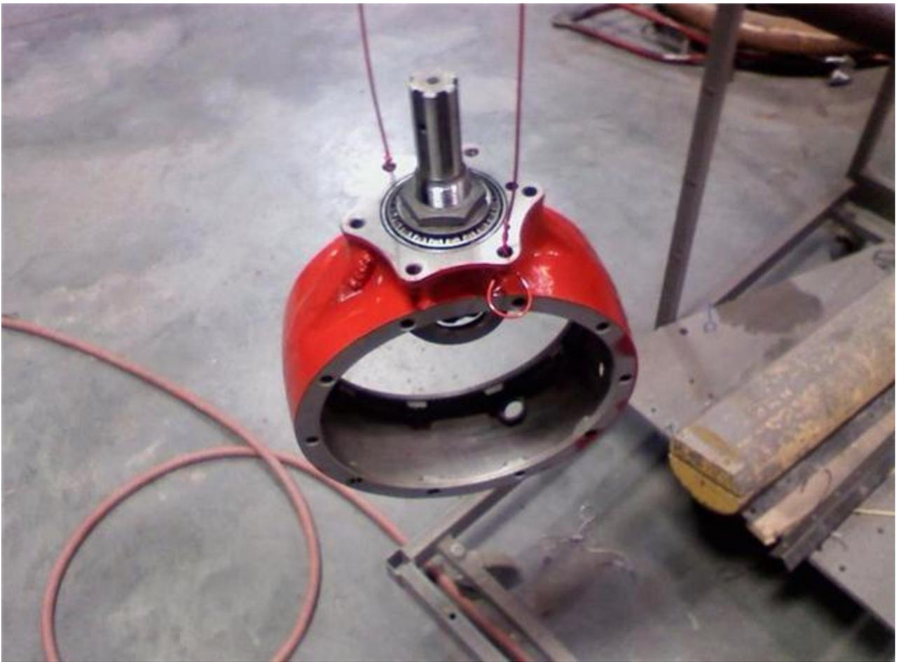
If you not going to powder coat you center section a torch will work. (Not cherry red) just some heat just like was needed to get the pinion bearing out. Still put the pinion assembly in the freezer. You may want to wait to paint you center after the pinion is installed. Don't want to burn the paint. I did take off all the over spray on the areas where the bells mount. Don't want it to interfere with my set up.
