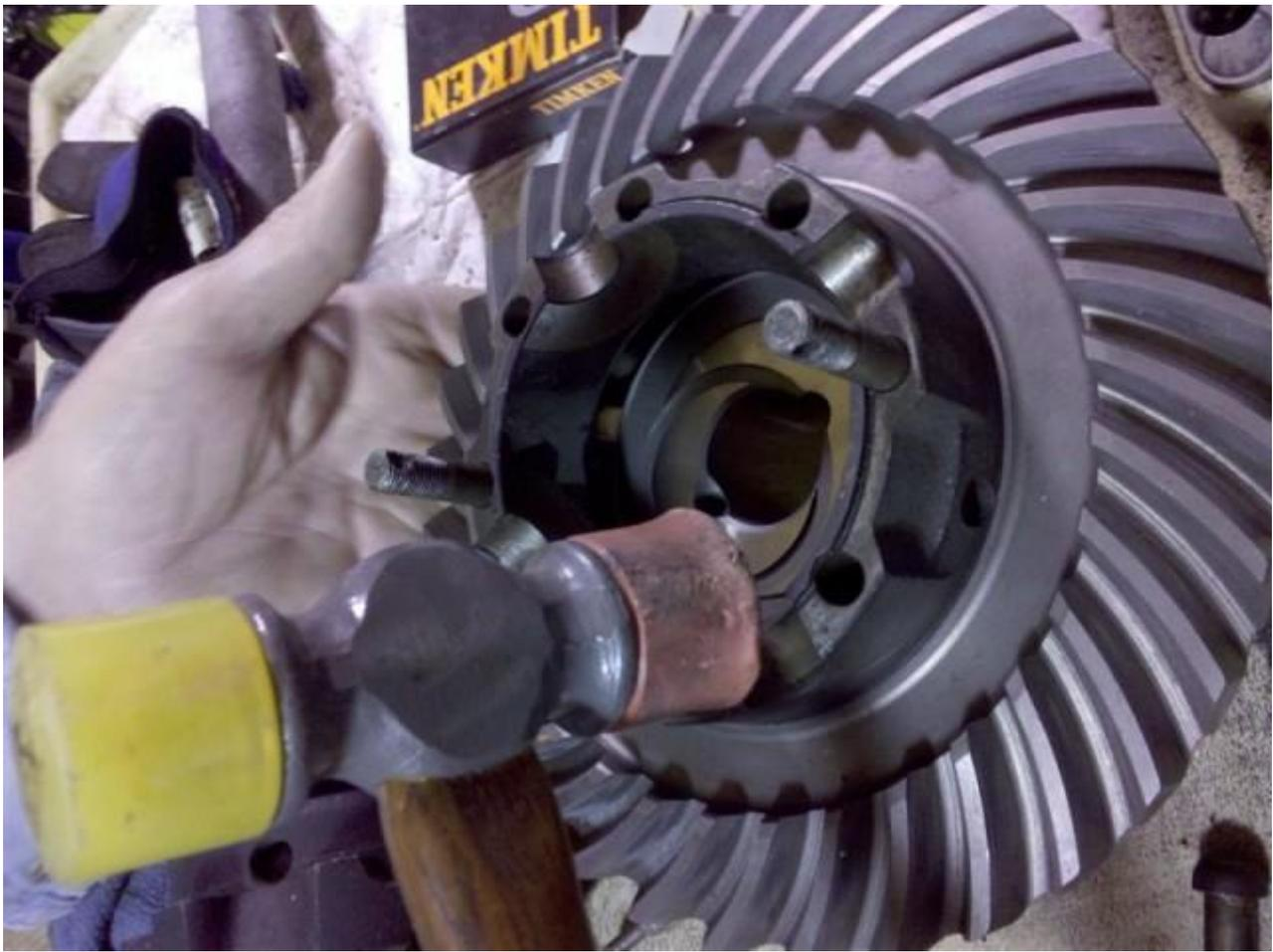
Then I set the other half of the diff (Big Half) with the bearing in place and set it in the vertical bell on the Cart. Slid an axle in it (Down into the bell) and placed the spider gears in the diff. I took a  $\frac{1}{4}$  nylon rope with a knot on each end. (Burnt the ends so it would not fray and untie). Total length measured about 5".
