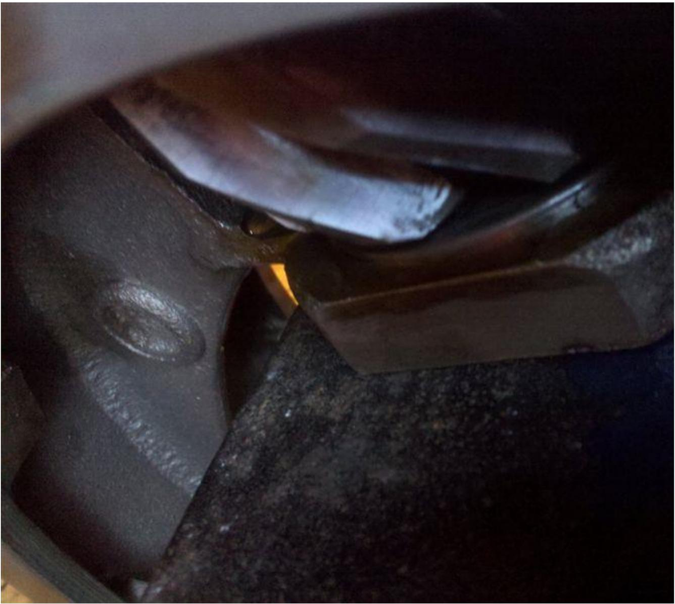
I put the retainer on and attached it in place with two 3/16 rivets.
