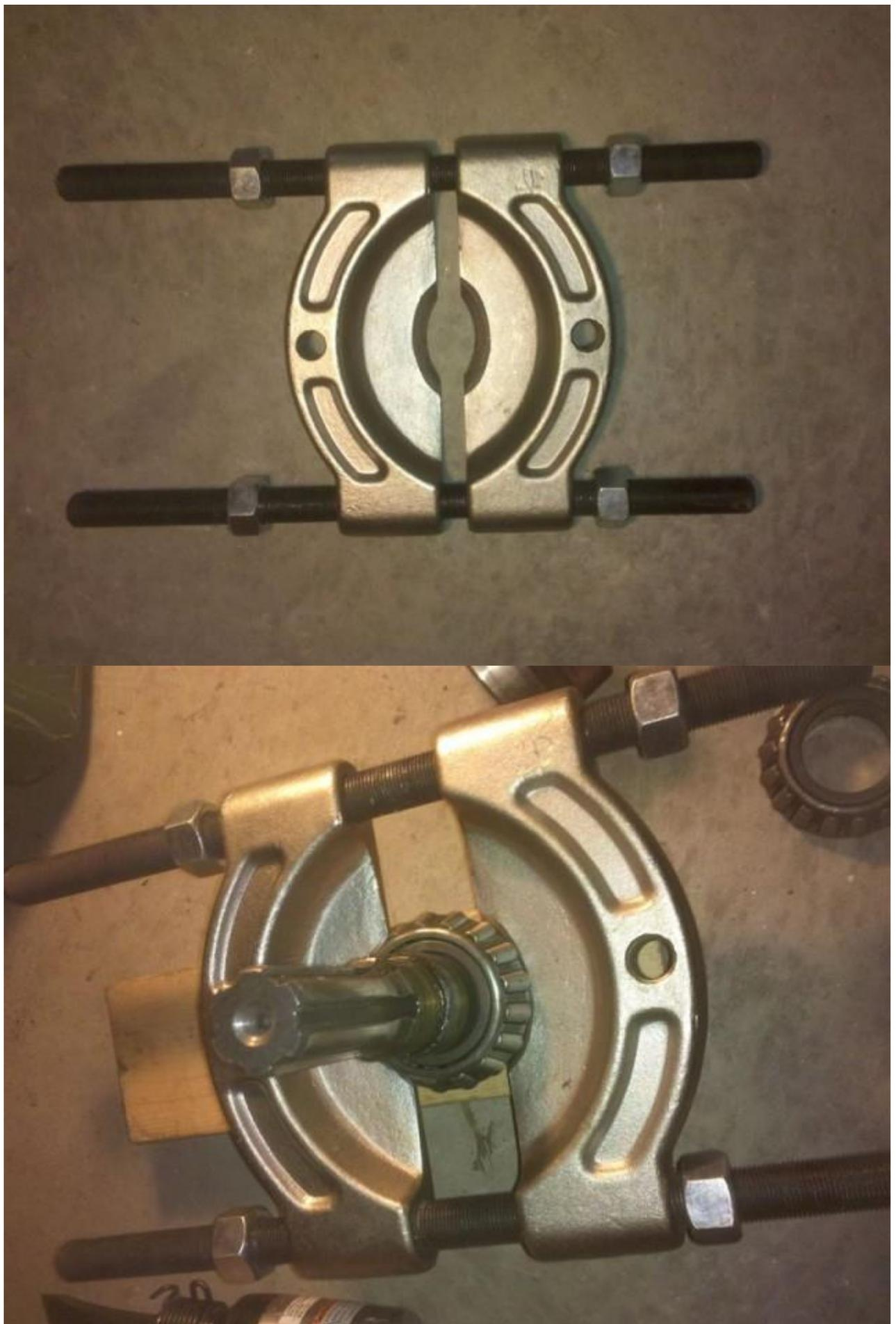
To remove a bad bearing: I cut the cage off with a cut off wheel and put a little heat on the race
