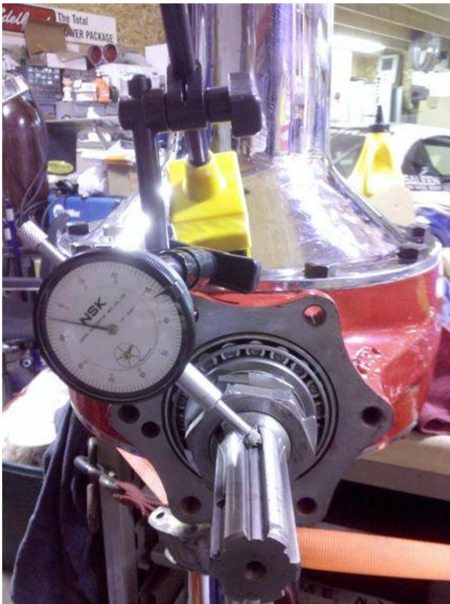
then I set it up to read from the Lock washer (That has not yet been bent over)and I got .016
