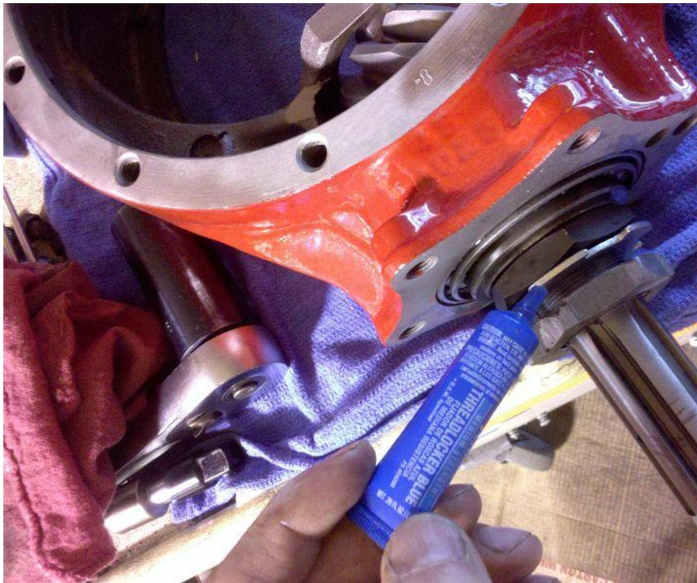
Because the lock washer had a pinion notch tab the first nut used to set preload will not spin when you tighten the outer nut. So you preload should stay the same as you tighten the out nut. Make sure to check preload when finished tightening.
