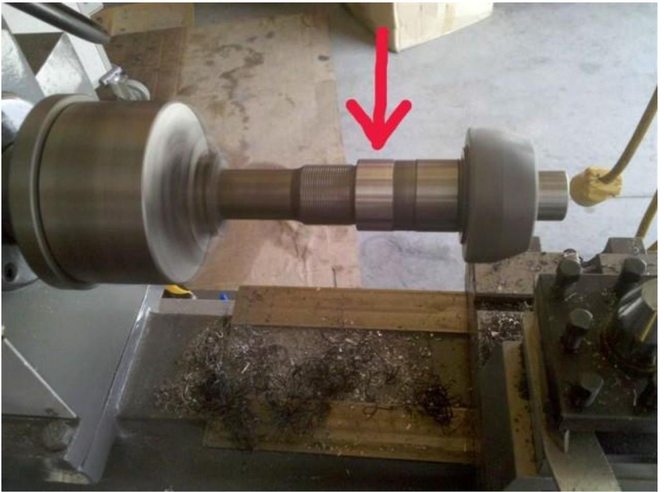
This could have been done by hand with some emery cloth but it was much faster chucking into my small lathe. I would take some material off with emery cloth and check. This was back and forth process. As soon as the bearing would slide I was good. You do not want to take too much off. Then it was time to press on the bearing on the gear end of the pinion. Using an old bearing race a piece of pipe and some gear oil I pressed it on.
