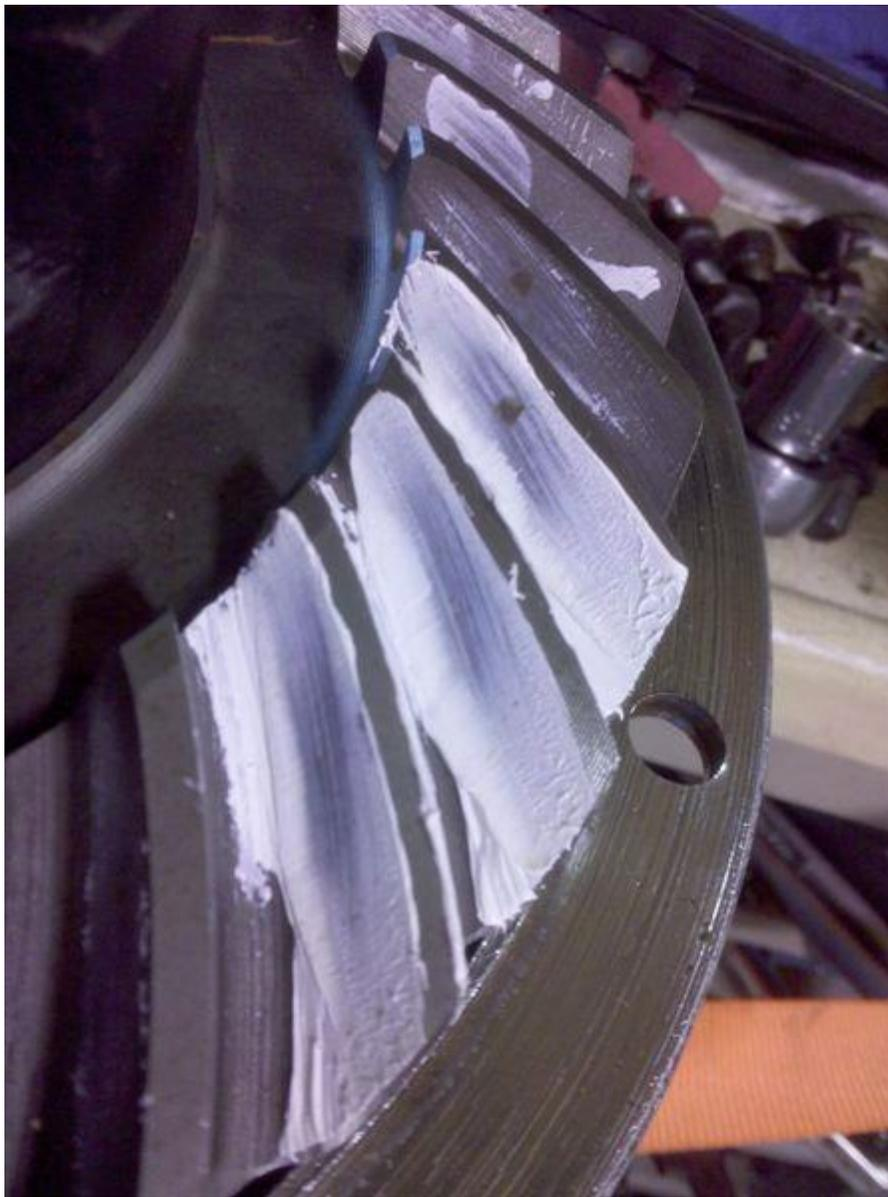
The pattern looked great. You don't want to see the pattern run off the ends at the toe or the heel of the drive or the coast side if you do. It will most likely howl. Either on acceleration or on deceleration depending if runs off the drive or the coast side.
