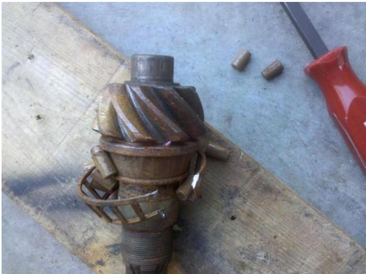
Remove the bearing on the None ring gear side of the differential: Just use the bearing splitter to catch the back side and get in the press. . I used a deepwell socket to go between the press and the diff. If saving the bearing no heat. If the bearing is junk, cut the cage and get some heat in it.
