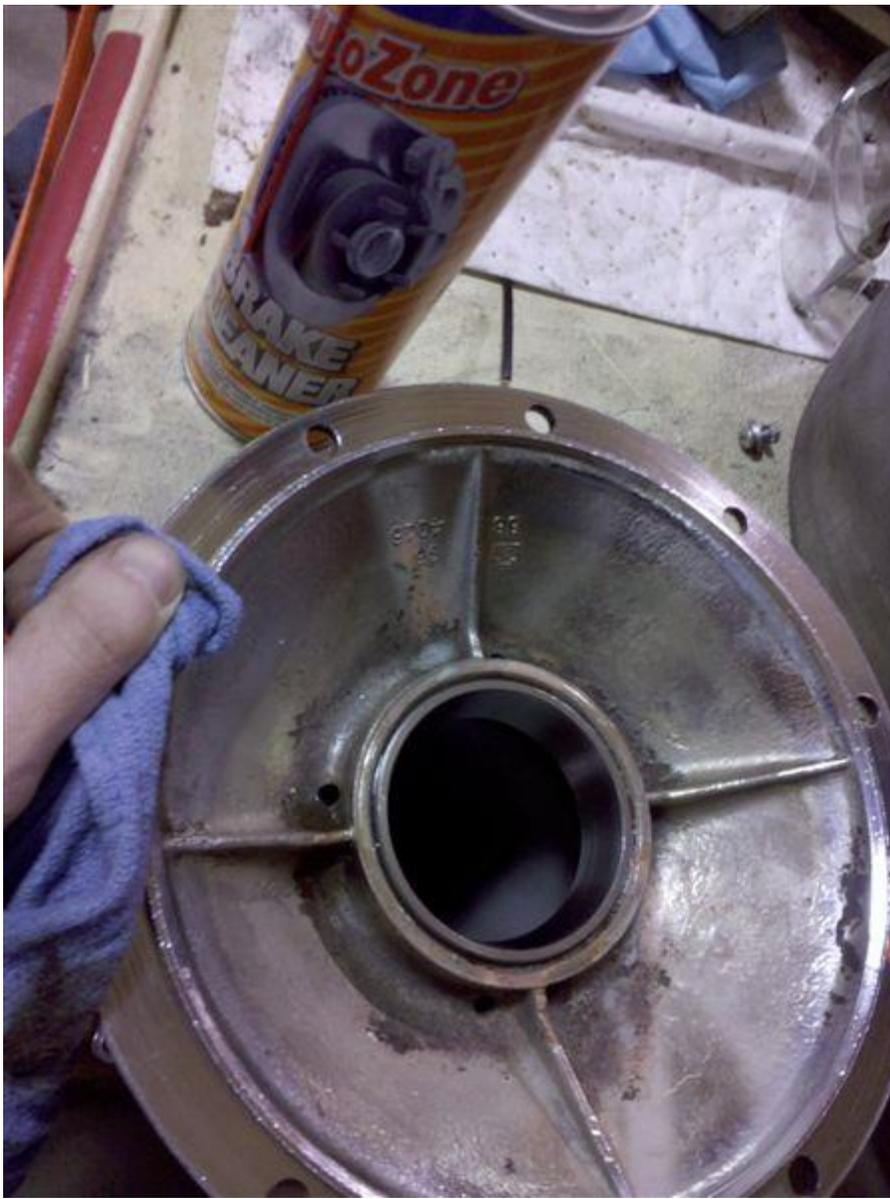
Bolt the center section to the bell with no gasket.
