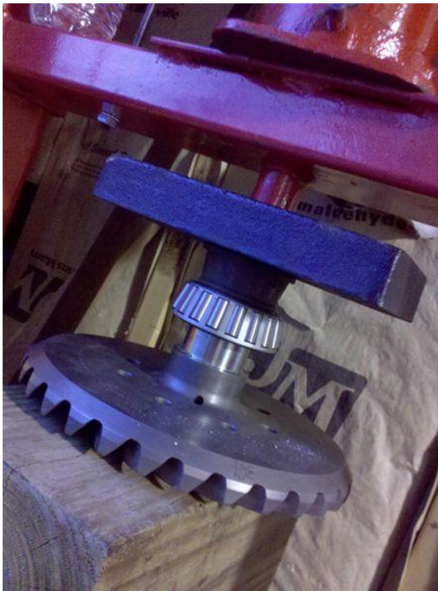
Then I repeated the above steps to press the bearing on for the big half of the diff.
