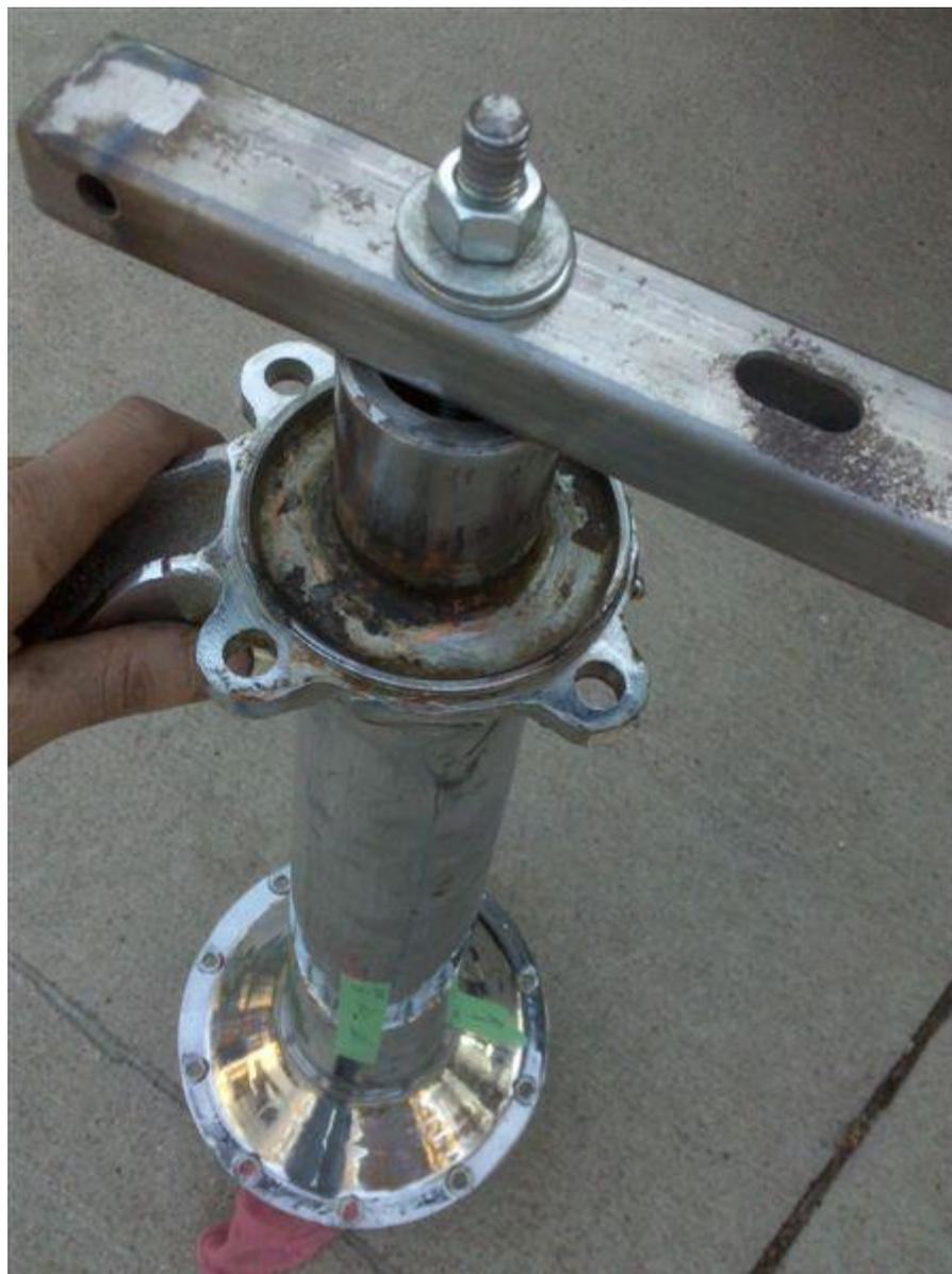
I put a bead of silicon sealant on the bells I went with a small bead because I did not want the sealant to interfere with my preload settings. When I put the gasket on I squeezed it up around the gasket to the top side of the gasket so silicone would be on both sides of the gasket. Geez this is taking me a long time to type. Almost done.
