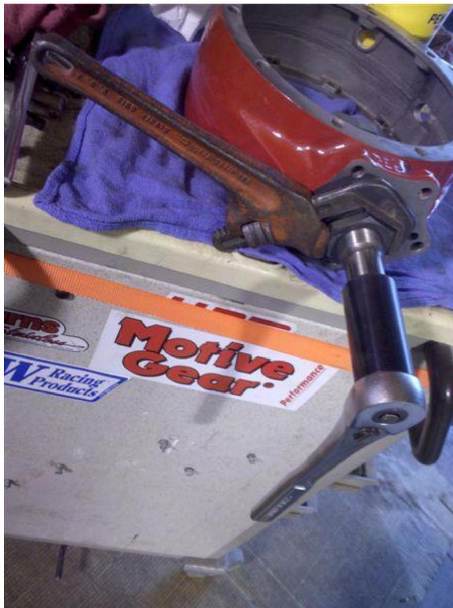
And check with my inch pound torque wrench. Till I got between 16 – 28 in lbs (new bearing specs) used bearings would be less. I ended up with 27 in lbs. then I tighten up the last big nut I used lock tight on the threads.
