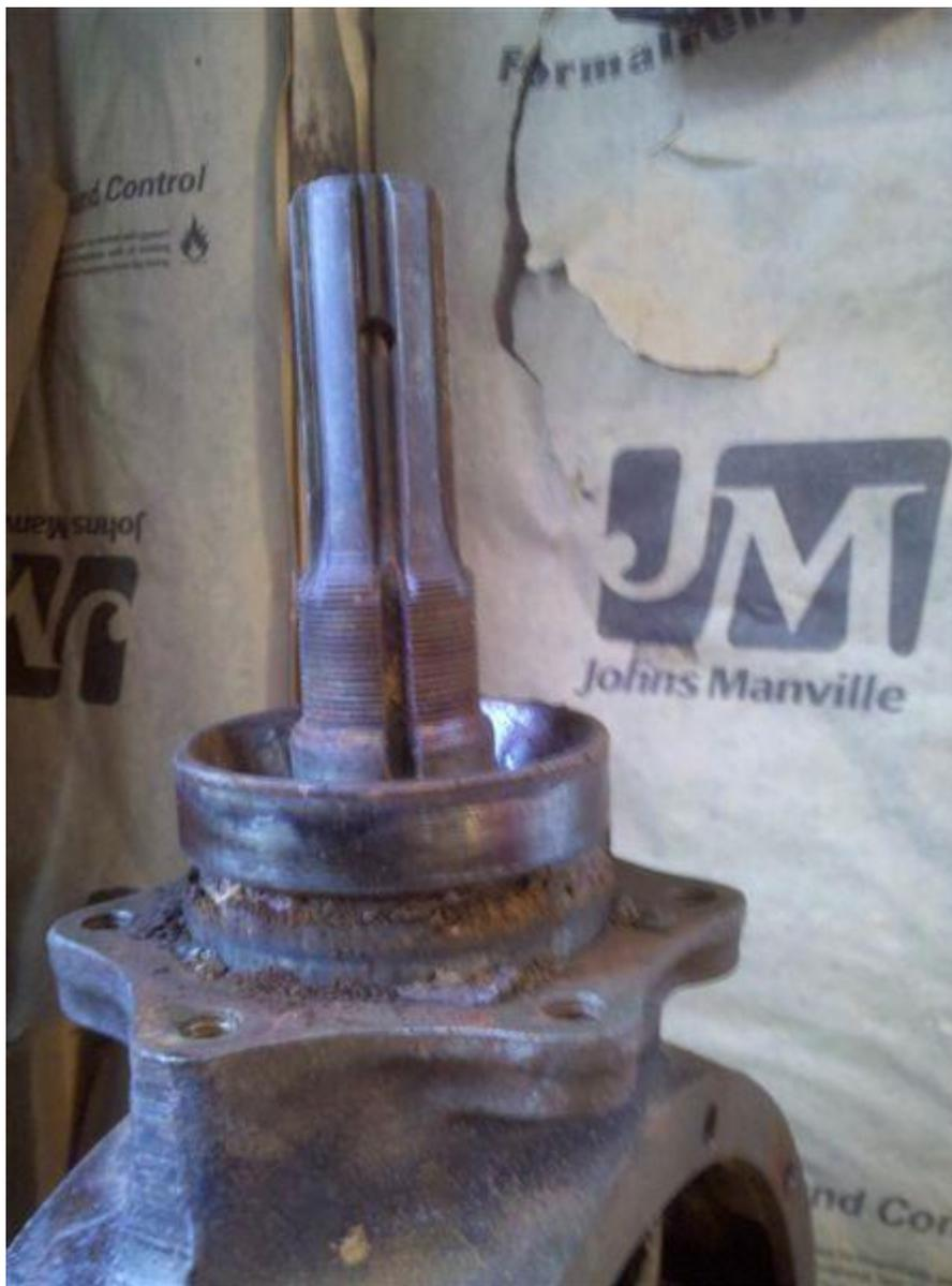
Next order of business was to get the pinion snout bearing out. If the rear end has not seen lot moisture or a failure where a bunch of shavings and chunks of metal have run through the bearing via the fluid. I would say this bearing could stay in place if the rollers look good. In my case I am planning on have the Center section (Banjo Portion) powder coated. I needed to the have the case completely gutted.
