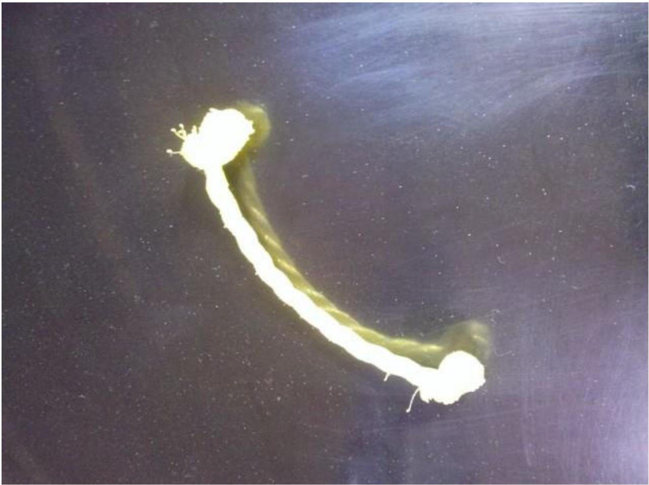
Took the knots and wedged them in between the spider gears and the axle end. Make sure this does not hold up the spider gears from fitting down in the correct position. This rope will temporarily lock the one axle into the diff while I set the preload on the diff bearings.
