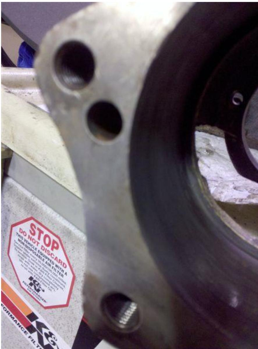
Josh and Jeremy up at trails powder coating took care of my while the pinion was put into the freezer and the banjo was masked to keep powder out of the insides and out of all bearing races and bell attachment areas. After two coats of kick ass red powder the center section was removed at 400 degrees and the cold pinion assembly with a skim coat of oil was slid right into the hole while it still hung from the wires. UUUUNG! Talk about a pretty site!
