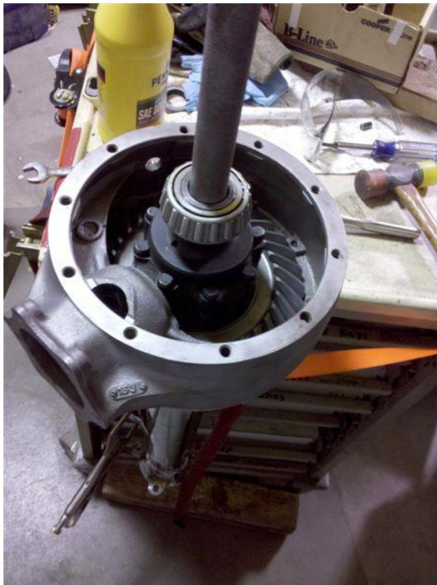
Now slide the other bell over the axle (Do not use gaskets at this time) and put about 4 bolts in to get it square and measure the gap. My gap measured about .020. So I took the bell off and I placed three gaskets shims .007, .007 and .005 back on the center section and bolted the bell back down tight.
