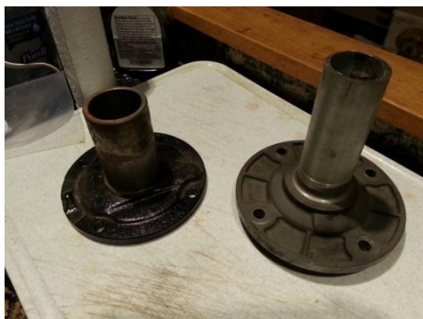
Flathead Bearing Retainer on left and T5 on right
