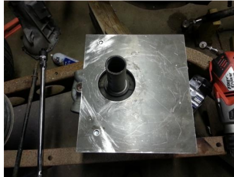
Plate after machining setting on hogshhead with Flathead Retainer (mark Retainer hole pattern - 4 places and hogshhead hole pattern – 6 places)
