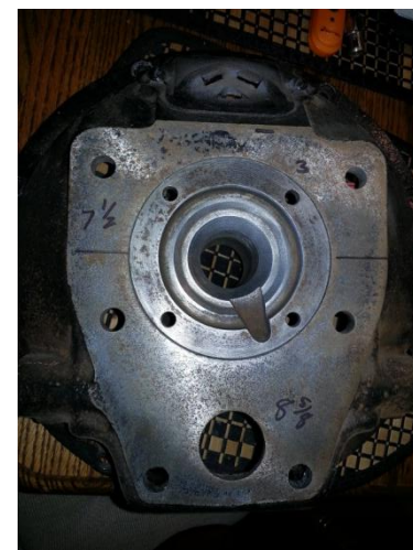
Flathead Bearing Retainer inside Hogshead
