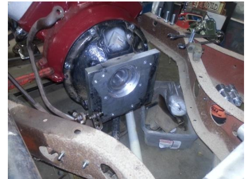
T5 Transmission pattern marked on Adapter Plate
