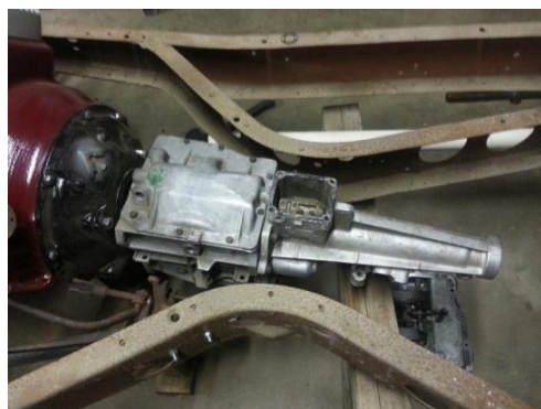
Ford T5 with S10 Tailshaft mockup in 33 Frame
