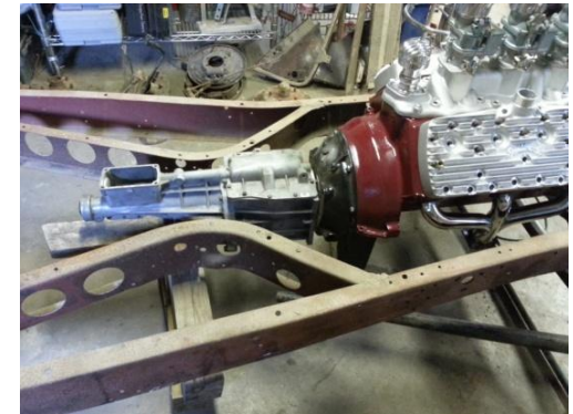
Ford T5 mocked up behind 59a Flathead and 34 Ford Frame
