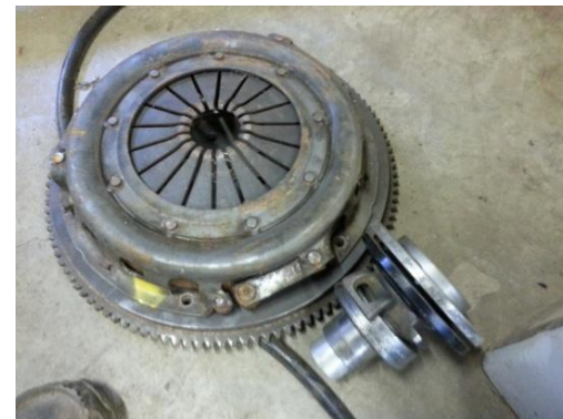
Mustang Pressure Plate and Flathead Retainer with T5 Retainer shoved inside and Flathead Throw-out Bearing and Hub
