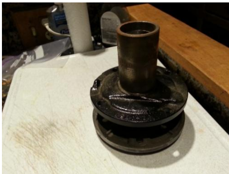
T5 Bearing Retainer inside of Flathead Retainer, Flathead Retainer honed to accept T5 Retainer
