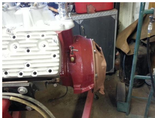
Hogshead mounted on 59a Flathead
