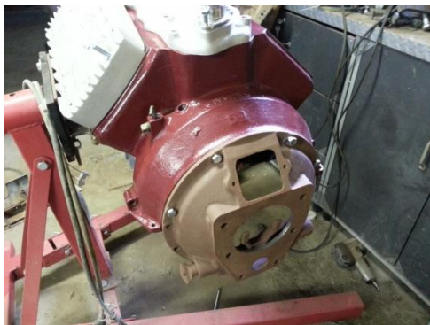
Hogshead mounted on 59a Flathead
