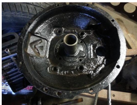
T5 Bearing Retainer inside of Flathead Retainer, Flathead Retainer honed to accept T5 Retainer
