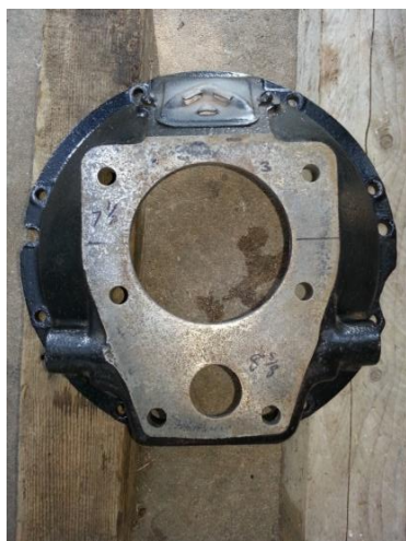
Hogshead Transmission mounting surface (6 bolts)
