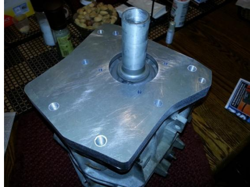
Adapter plate on T5 Transmission with T5 Retainer
