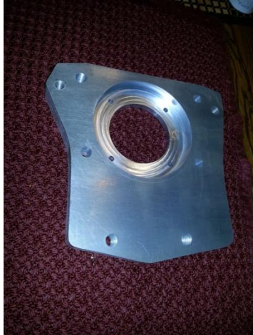
Adapter plate cut to T5 outline, 4 flathead Retainer holes cut and taped, 6 hogshhead holes cut and taped, two upper T5 holes cut and taped.
