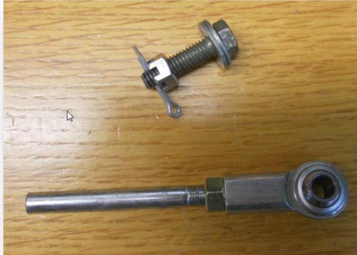
Take your 1/4" bolts and file 1/4" of the end so it's a round cylinder. The diameter will be the width of the groove in your pedal pivot shafts. It should be roughly the minor diameter of the bolt but may vary depending on how much wear your pivots have. You can test fit these holding bolts in the pivot point to make sure they are not binding as the pedal arms are moving. File the ends of the bolts to a point where no binding is felt.
