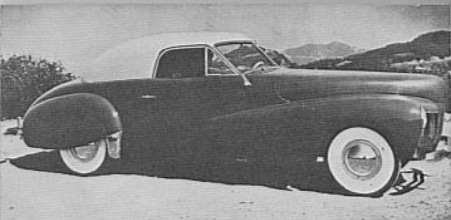
Another Coupé 66 Ville is shown here on a 1941 Mercury chassis. Note how the body has been lengthened for greater wheelbase by increasing the depth of the cowl section—between the dashboard and hood bonnet...
